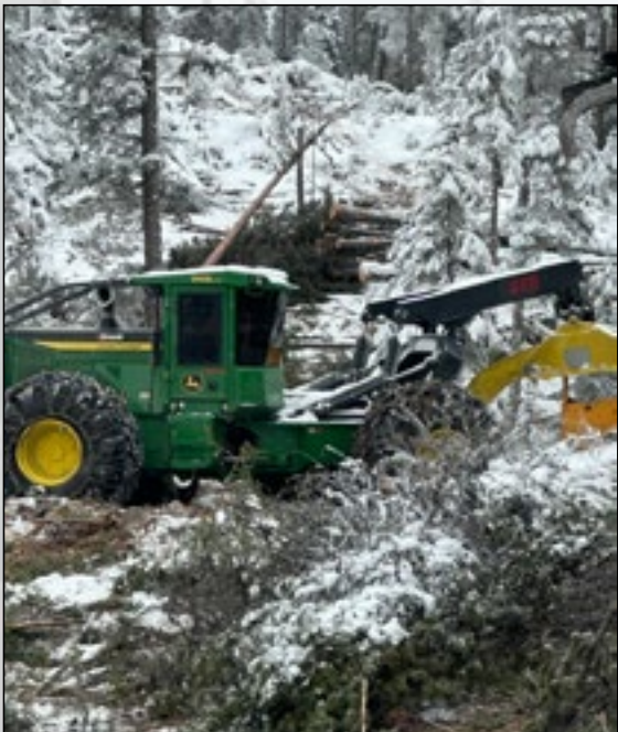
SFE skidder skidding a bunch of felled timber to roadside where it will be processed.
