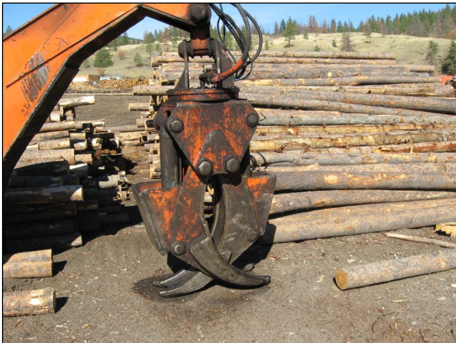
Photo 10. View of a buncher located on the southern portion of the Plan 59794 Post Mill facing northwest. Note the leaking hydraulic oil and soil staining.
