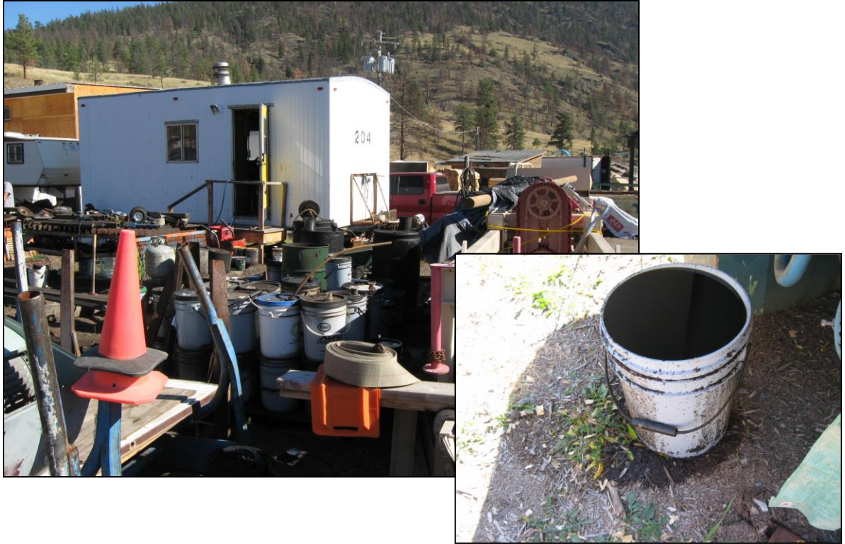
Photo 3. View of the hydrocarbon storage on the west side of the of the travel trailers in the northwest portion of the Site (Plan 59794 Post Mill) facing northeast. Note that many containers are open, overflowing, and the entire area contains spotty soil staining.
