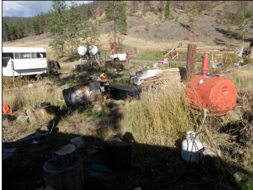
Photo 15. View of the Lot 297 ASTs facing northeast. Note the two 1800L ASTs (Diesel and Gas) on the left, the rusted 800L tank (unknown), and the red empty tidy tank.
